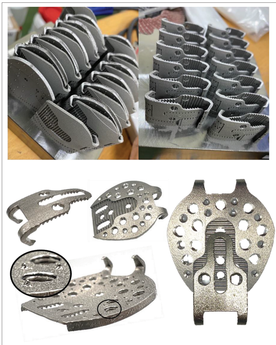
Figure 4. (a) 3D-printed AATBP prototypes without screw/wire holes and (b) 3D-printed AATBP with back cone bump after screw/wire holes generation by CNC machining.
