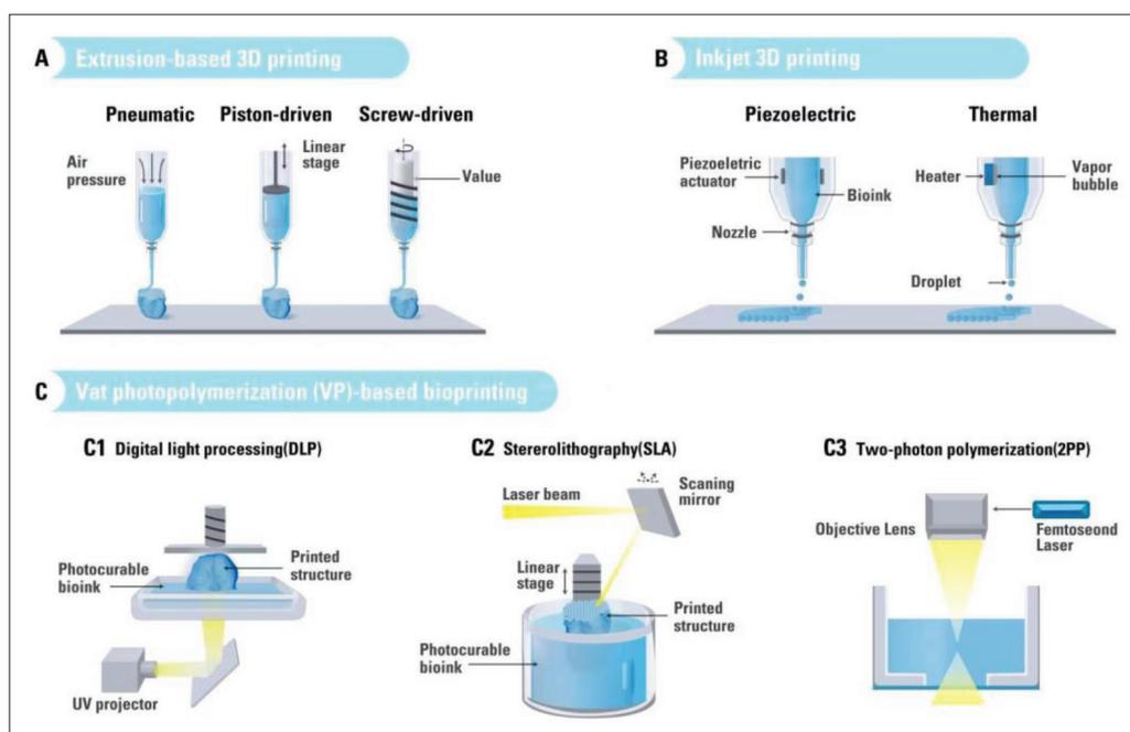
**Figure 5.** Representative demonstrations of 3D bioprinting methods. (A) Extrusion-based 3D printing; (B) Inkjet 3D printing; (C) Vat photopolymerization (VP)-based bioprinting: C1, digital light processing (DLP); C2, stereolithography (SLA); C3, two-photon polymerization (2PP)<sup>[61]</sup>.
