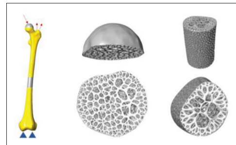
Figure 14. Bionic bone scaffolds for femoral defect site.
